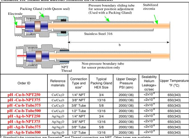
$<sup>^</sup>st$  Standard tube connectors are Swagelok $^ extstyle{ ilde{8}}$  and Thread connectors are NPT. Other types are available.
